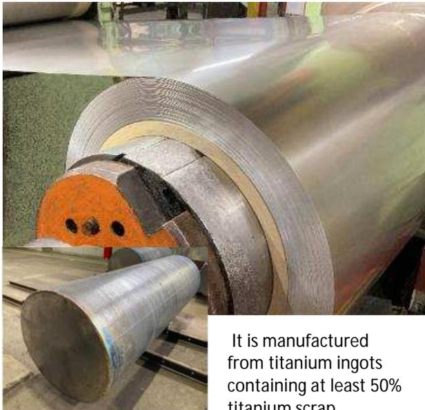
It is manufactured from titanium ingots containing at least 50% titanium scrap.
